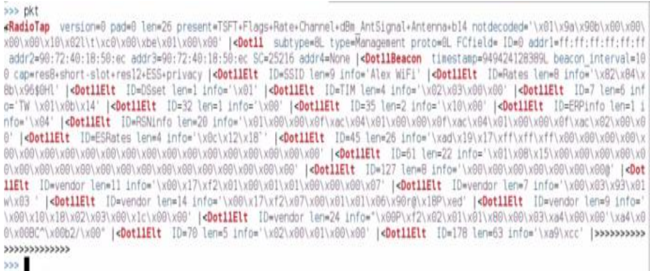
Figure 5. Showing a packet caputed through scapy
