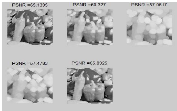
Fig 9: Dilation on Pepper image using different structuring elements (disk, square, diamond, line, rectangle)
