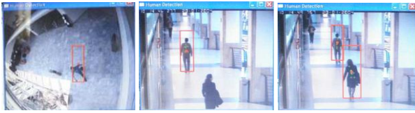
Fig. 6 (a) Human detection for upside camera (b) Human detection from front side camera (c) Multiple human detection
