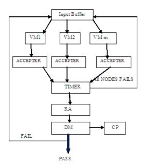
Fig 1: Proposed Fault Tolerance system
