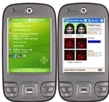
Fig. 5. HTC P3400 Running Developed Application for Face Recognition
