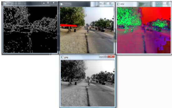
Fig 8: Misdetection of Hough Transform based Conventional Techniques due to improper markings
