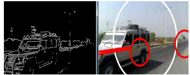
Fig 18: Successful boundary detection even when a vehicle is crossing the sight of the boundary
