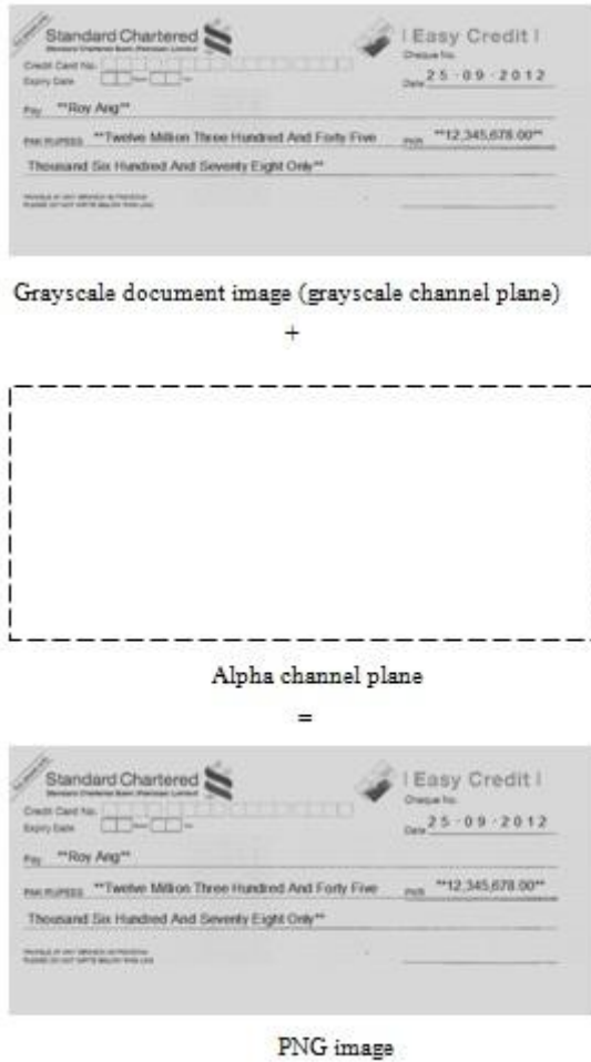
Fig 1: illustration of creation of a PNG image from a grayscale document image and an additional alpha channel plane
